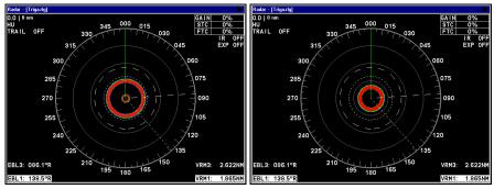
Before adjusting the Trigger Delay for 4 kW radars, two rings will be shown on the screen (left). As Trigger Delay is increased, the larger ring will start to get smaller. The small ring will disappear (right).
